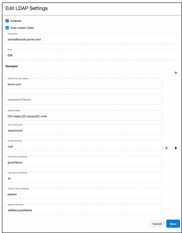
The following example requests enable LDAP authentication over SSL with an Active Directory server at address **activedirectory.company.co** using the **us.company.co** domain:
