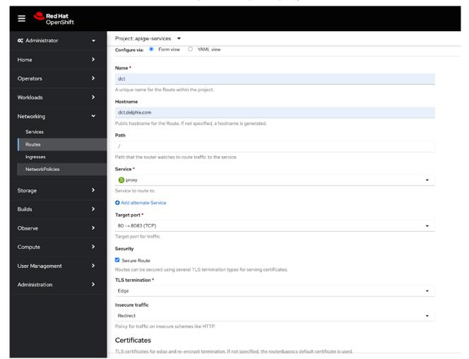
If SSL is not terminated at the Route level, then create a PassTrough route and use 443 port of the proxy service, and configure the SSL certificate and key in the values.yaml file:
