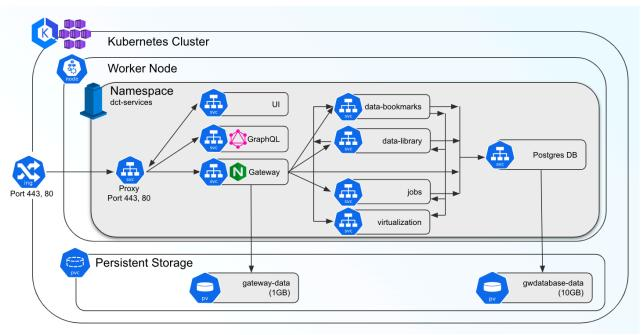
DCT is multi-cloud enabled, which means that a single DCT instance can be deployed to orchestrate (via HTTPS) Continuous Data and Continuous Compliance workloads with Delphix engines located in other networks. Alternatively, DCT can be localized to engines located within a network. DCT is a lightweight management application, which means that it does not require a highly performant connection to complete its work and can serve as a central management layer for Delphix engines globally.
