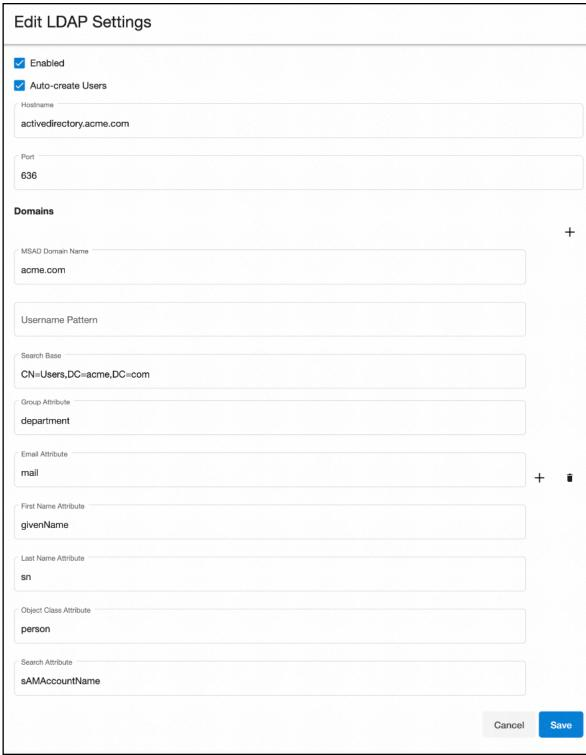
The following example requests enable LDAP authentication over SSL with an Active Directory server at address activedirectory.company.co<sup>32</sup> using the us.company.co<sup>33</sup> domain:
